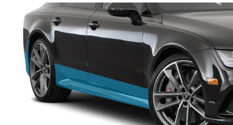
ROCKER PANELS & REAR WHEEL IMPACT AREA
