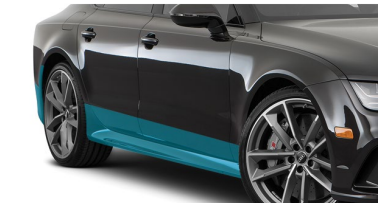
ROCKER PANELS & REAR WHEEL IMPACT AREA
