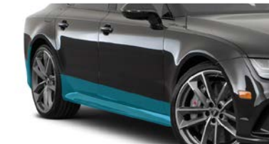
ROCKER PANELS & REAR WHEEL IMPACT AREA
