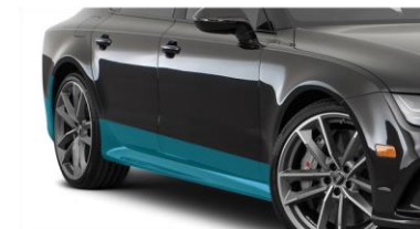
ROCKER PANELS & REAR WHEEL IMPACT AREA
